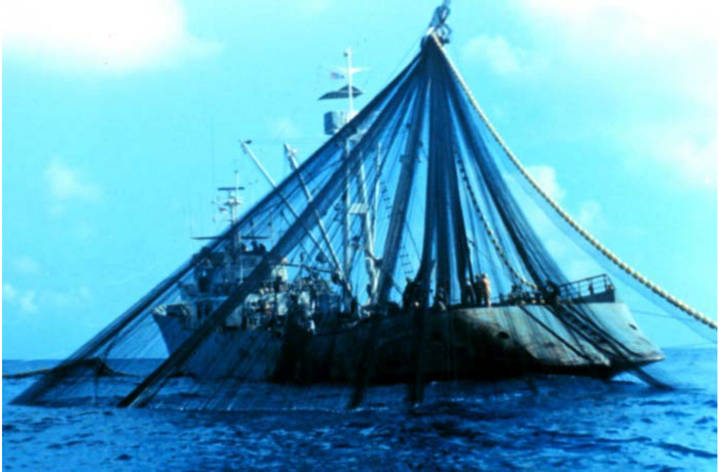
After closing the net and trapping the fish, the net is now brought on board. This is a view of the net being run through the powerblock and then laid back on the stern of the fishing vessel. Image ID: fish2146, Fisheries Collection
